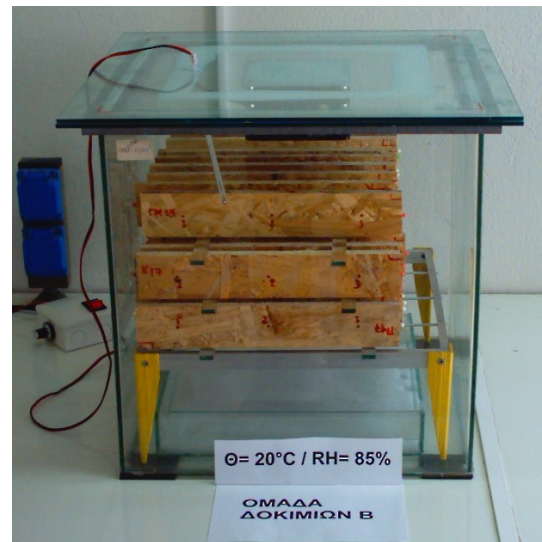
Figure 3. Conditioning chamber containing specimens
