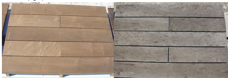
Figure 2: Furfurylated Maple wood deck: (left) as in May 2011 and in May 2014 (right)
