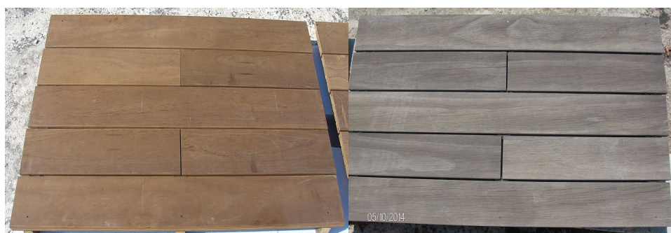
Figure 1: Furfurylated Radiata pine wood deck: (left) as in May 2011 and in May 2014 (right)
